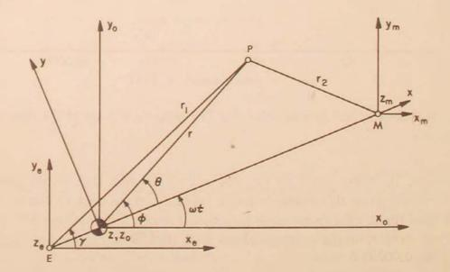
Figure 4. Coordinate systems. E, earth; M, moon; P, particle.
