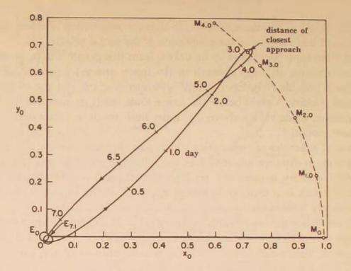
Figure 17. Return to hit the earth after passing near the moon—direct motion (r = 4300 miles;  $\phi = -90$  degrees; V = 34,850 ft/sec;  $\gamma = 19.25$  degrees). E, earth; M, moon.
