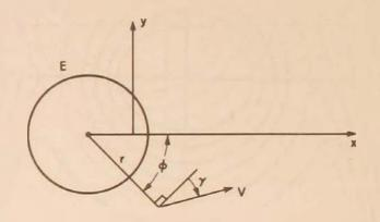
Figure 8. Parameters used to describe initial conditions. E, earth.
