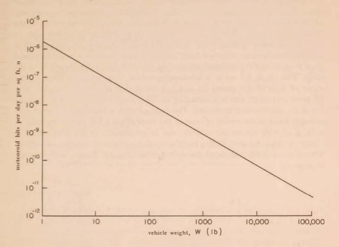
Figure 3. Frequency of hits by meteoroids that will impart a velocity of 0.1 ft/sec or more to the vehicle.
