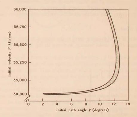
Figure 11. Initial conditions for lunar impact (r = 4300 miles;  $\phi = -112.5$  degrees).
