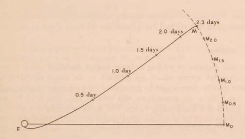
Figure 12. Moon-rocket transit trajectory—impact (r = 4300 miles;  $\phi = -108$  degrees; V = 35,000 ft/sec;  $\gamma = 14.2$  degrees). M, moon; E, earth.
