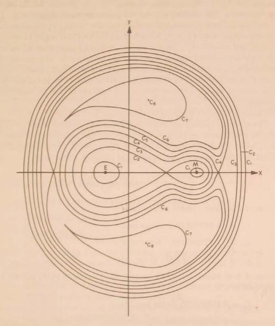
Figure 5. Contours of zero relative velocity in (x, y) plane. E, earth; M, moon.
