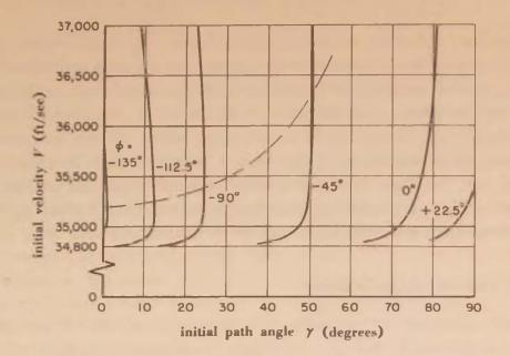
Figure 9. Initial conditions required to hit the moon-direct motion.
