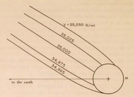
Figure 13. Effect of varying V on impact location (r = 4300 miles;  $\phi = -108$  degrees;  $\gamma = 14.2$  degrees). M, moon.
