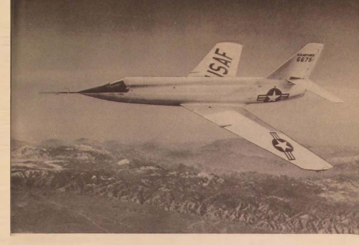
The Bell X-2, powered by a Curtiss-Wright liquid-fueled rocket engine with 15,000 pounds thrust, reached an altitude of some 126,000 feet, just under 24 miles, and a speed exceeding 2000 mph at about 70,000 feet, in two flights in September 1956. This swept-wing aircraft weighed 18,000 pounds, had a wing span of some 32 feet, and a length of 37 feet. The X-2 was air-launched from a B-50 carrier.
