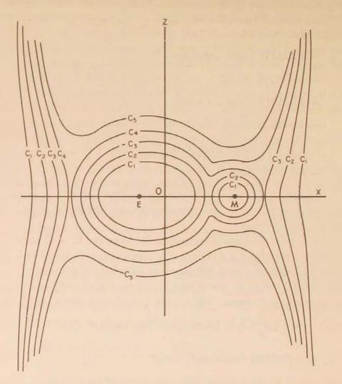
Figure 6. Contours of zero relative velocity in (x, z) plane. E, earth; M, moon.
