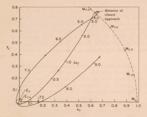
Figure 16. Return near the earth after passing near the moon—direct motion (r = 4300 miles;  $\phi = -90$  degrees; V = 34,825 ft/sec;  $\gamma = 17.0$  degrees). E, earth; M, moon.
