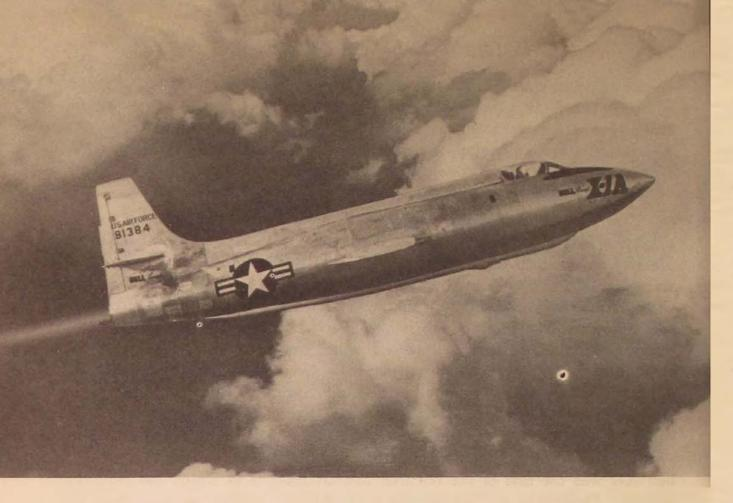
The Bell X-1A, approximately five feet longer than the X-1, weighed about the same and was powered by the same engine as the X-1 but modified to afford some 4.2 rather than 2.5 minutes of powered flight. It was flown at a speed of 1650 mph at an altitude of about 70,000 feet in December 1953; and in May 1954 a height of 90,000 feet was reported. Both the X-1 and the X-1A were air-launched from a B-29.
