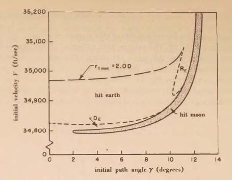
Figure 15. Initial conditions to return to earth (r = 4300 miles;  $\phi = -112.5$  degrees).
