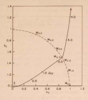
Figure 14. Transit trajectory—escape from the earth (r = 4300 miles;  $\phi = -112.5$  degrees; V = 35,000 ft/sec;  $\gamma = 12.3$  degrees). M, moon; E, earth.
