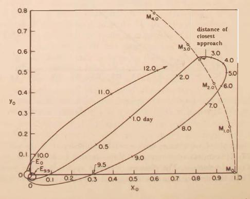
Figure 18. Return near the earth after passing near the moon—retrograde motion (r = 4300 miles;  $\phi = -90$  degrees; V = 34,950 ft/sec;  $\gamma = 22.0$  degrees). E. earth; M. moon.
